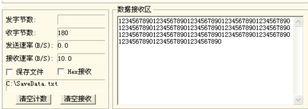
After the connection is established, PC-B will continue to receive data and send data to eth0 through the network debugging tool.
